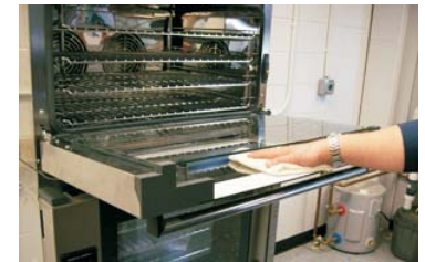
2. Clean back of outer door glass & front of inner door glass.*
