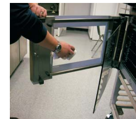
2. Clean back of outer door glass & front of inner door glass.*
