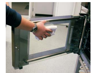
3. Swing inner door glass forward until top & bottom glass holder clips click & hold glass. Clean back of inner door glass.*
